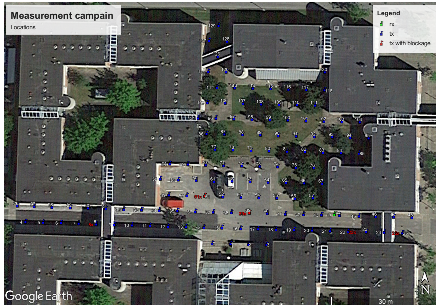
Figure 1.2: The green square is the location of the receiver, the blue squares are the location of the transmitter without the metal plate in front, and the red squares are the transmitter locations with a metal plate in front. The figure is from [19].
